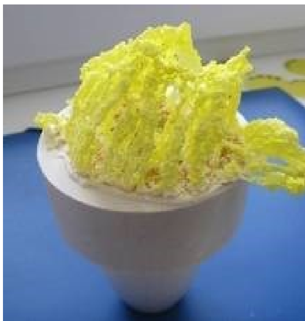
Figure 1. Synthesized YAG:Ce sample: a – fibers on crucible lid; b – SEM-images of agglomerated powder.
